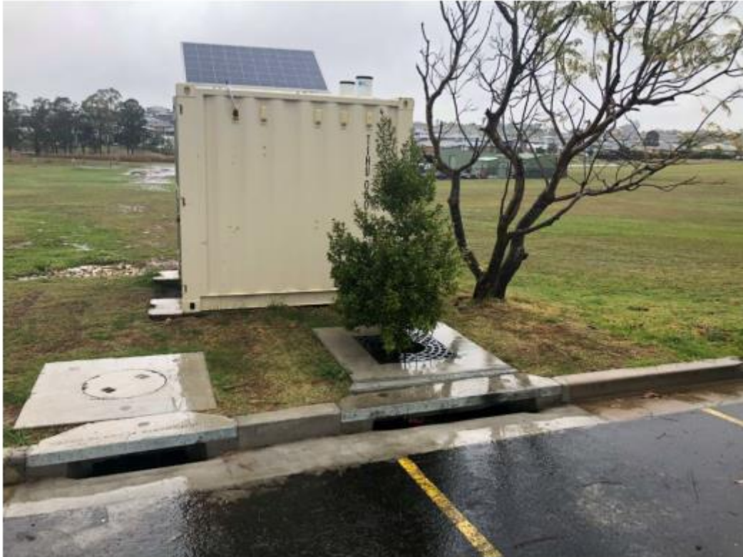
Figure 5: Side Entry kerb and sampling facility at Kingswood Campus, Western Sydney University
