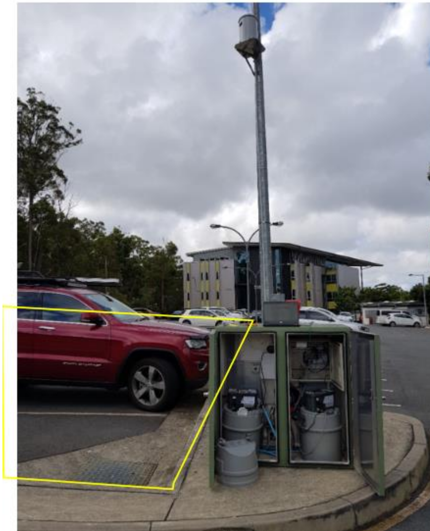
Figure 4: Showing the Atlan Stormsack monitoring equipment and the catchment behind in yellow.
