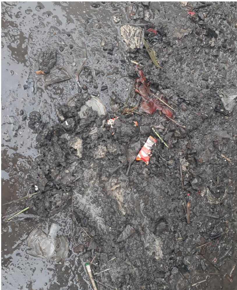
Figure 6 - Photos of captured gross pollutants confirming most material is sediment and organic material
